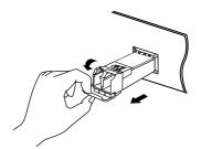
4. Reinstall the protective dust plug in the transceiver's optical bores and place it on antistatic mat or a static shielding bag.
